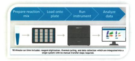
Figure 2. The Absolute Q platform workflow. DNA, primers, and probes are added along with reagents. Next, samples are loaded onto plates that can accommodate up to 16 samples at a time. Then, plates are loaded onto the QuantStudio Absolute Q system where droplets are generated by microfluidic array plate (MAP) technology and the dPCR reaction is then run. Finally, QuantStudio software performs mutation detection and quantification with precision and confidence.
